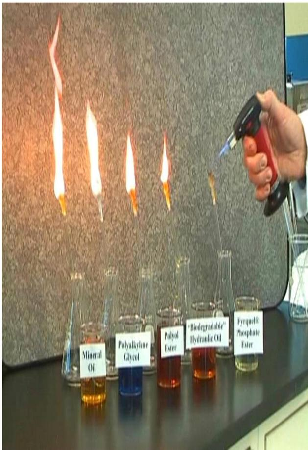
This may come as a surprise but some so called fire resistant fluids are imposters. They do not provide the basic threshold characteristics for fire resistant fluids, that is, not sustaining combustion and remaining difficult to ignite during service. These ISO Class HFDR fluids are easily shown by standard fire tests like the hot manifold ignition ISO test to be not self extinguishing.
